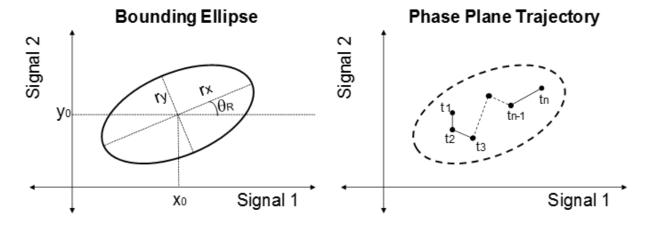
The X-Y plane is the phase plane defined by the two signals.  $r_x$  and  $r_y$  are the radii of the bounding ellipse along the x and y axes, and  $\theta_R$  is the rotation of the ellipse about the center. The ellipse center is at  $(x_0, y_0)$ . In the image, the phase plane trajectory of the signals lies within the bounding ellipse for all time-points  $t_1$  to  $t_n$ .
